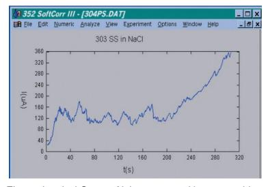
Electrochemical Current Noise generated by metastable pitting of 303 SS in 1000 ppm NaCl. Sample was held potentialstatically at 600 mV vs. open circuit.
